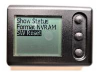
With OK highlighted, click the middle button once then immediately press and hold the top & bottom buttons for 5 seconds. (This will put the device into 'firmware update mode')
