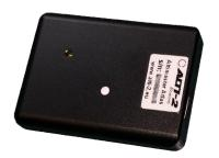
Insert Atlas into the helmet's audible pocket with the speaker hole facing inward (towards the ear). Failure to do so may result in inaudible alarms.
