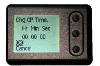
Use the top and bottom buttons to change the number of hours. Press the middle button to move on to minutes, and again to seconds.
