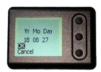
Press the middle button to scroll to and select **OK** to save the new time setting.
