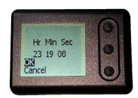
Press the middle button to scroll and select **OK** to save the new time setting.
