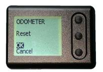
To reset the Odometer to zero, select **OK**.
