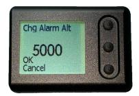
Use the top and bottom buttons to change the alarm altitude. Once you have the correct altitude, press the middle button to highlight **OK**.
