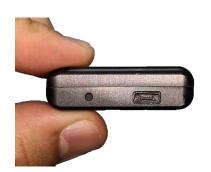
Gently insert the end of a paper clip, or similar thin utensil, press and hold the reset button for five to eight seconds.
