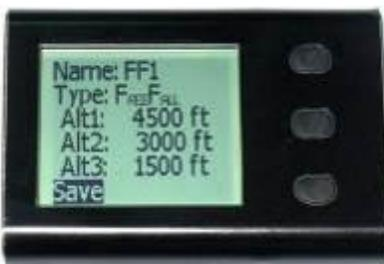
Repeat the process for the other Alarm Altitudes and once all values are set, scroll to and select **Save**. The new alarm settings are now active.
