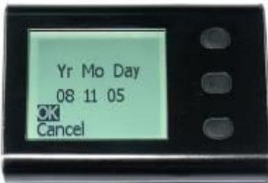
Press the middle button to scroll to and select **OK** to save the new time setting.
