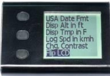
Using the **Flip LCD** function on the **Display Opt** menu, your N3 can be oriented with the buttons in either direction, on either side of your helmet.
