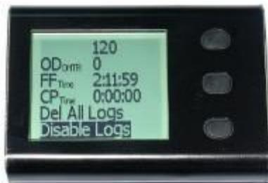
If logging is enabled, **Disable Logs** will appear at the bottom; otherwise, **Enable Logs** will appear.
