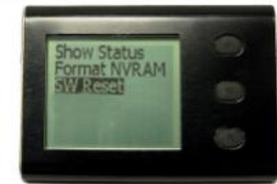
Select **SW Reset**, and then select **OK** to restart the main program. N3 will show you the **Alti-2** greeting screen, then the firmware version and unit serial number will appear. After a few seconds N3 shows the Ground Screen, and then the screen blanks. Press any button to bring the screen back into view.
