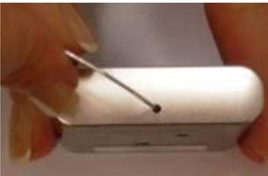
Gently insert the end of a paper clip, or similar thin utensil, press and hold the reset button for five to eight seconds.
